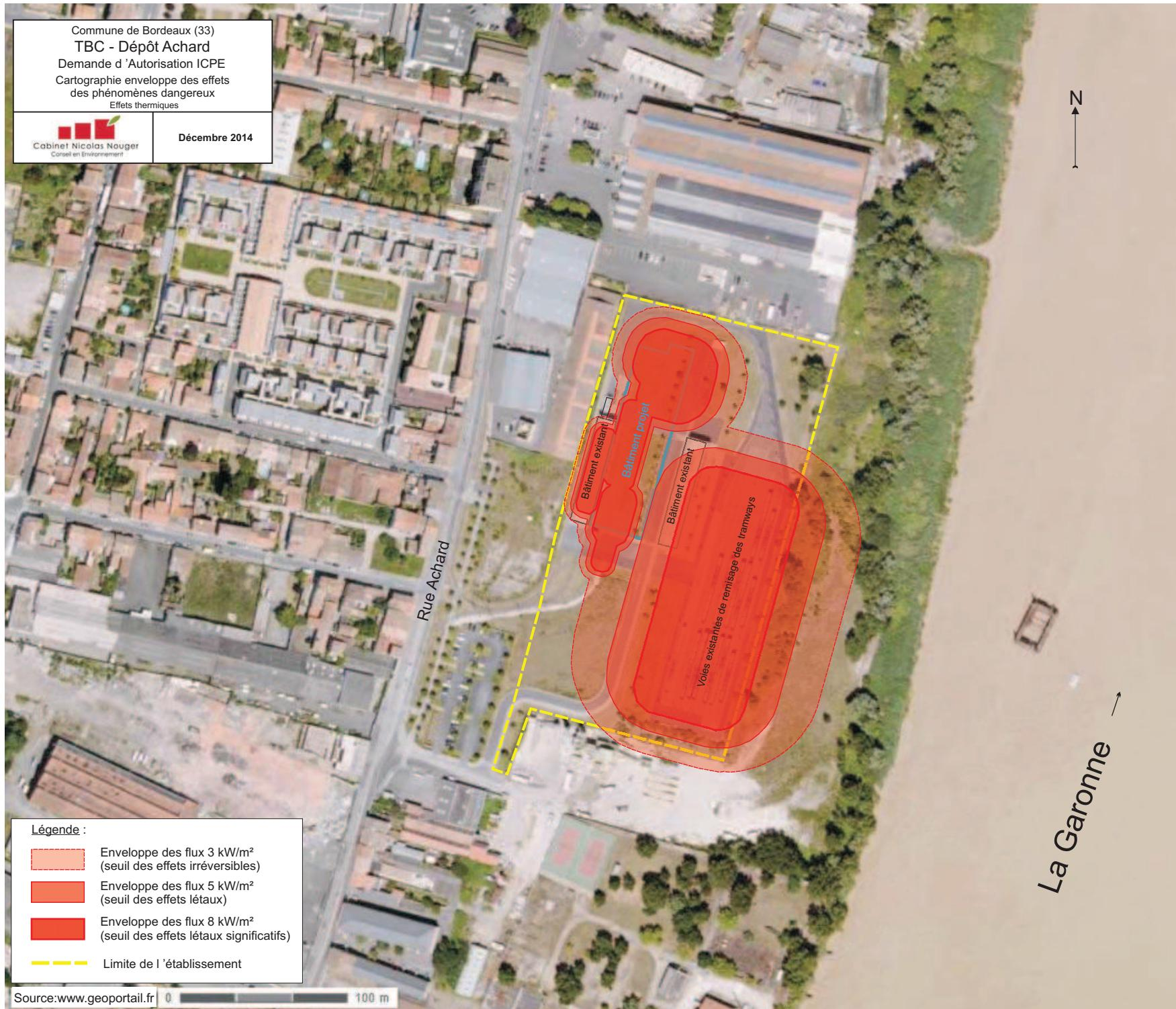
Planche PL1 - FLUX THERMIQUES - INCENDIE D'UNE RAME DANS LA CABINE
